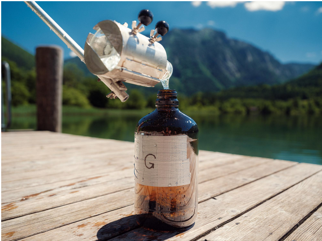
Figure 2: sampling equipment used, showing sample pole, 500ml sampling bottle and 2.9 litre composite sample container (Winchester)
